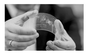
Are indispensable in the production of displays, monitors, touch screens and photovoltaic cells. Currently, the most commonly used TCFs are based on indium–tin oxide (ITO). Indium is a rare element whose supply on a global scale is mostly controlled by China (about 50%–60% of global production) and Korea (15% market share). ITO-based films are not flexible (which is a serious limitation for electronics manufacturers); they insufficiently conduct electricity
