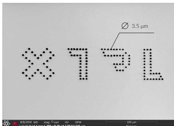
Fig. 2 Example illustrating the outstanding precision of the XTPL solution. Mircodots, used, for example, in the semiconductors and sensors sectors, now usually have a diameter of 50 \mu\text{m} (micrometers), but not less than 20 \mu\text{m} . By now, XTPL has managed to achieve structures of a mere 1 \mu\text{m} , while working on further reduction of this parameter.
